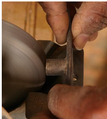
Clean up the casting. You'll need to remove the remains of pouring rods attached at the foundry. Use a hacksaw, and then flatten the base of the pull's post on a grinder or with a file.
